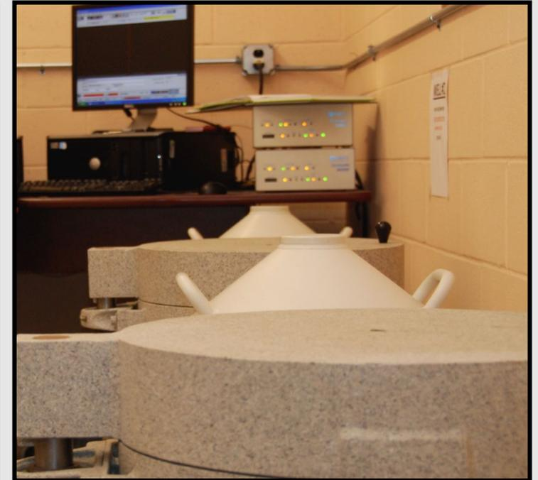
Intrinsic germanium well detector coupled to a multichannel analyzer
